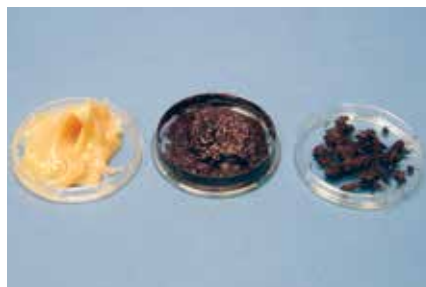
Fig. 6: From left to right: 1) new grease, 2) heavily oxidized grease, and 3) worn-out (failed) grease – the thickener and additives have decomposed and the oil is breaking down.
