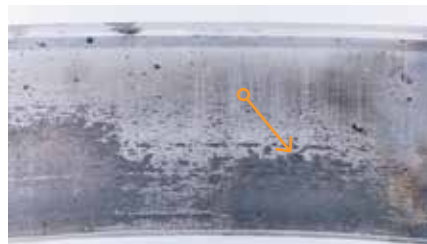
Fig. 13: Cylindrical roller flattened as a result of skidding.
