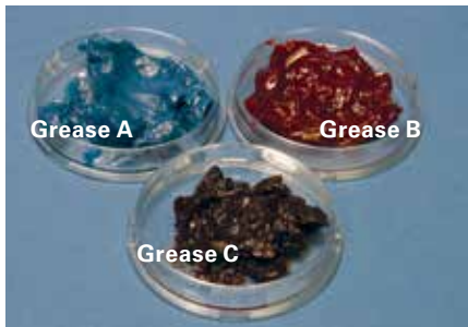
Fig. 4: Grease A and Grease B are not compatible. Mixed together they become lumpy, discolored and hard in composition (Grease C).
