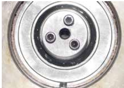
Fig. 1: Clean grease leaking slightly.
