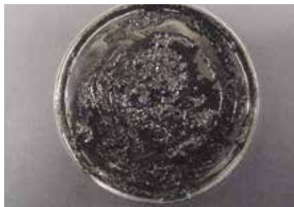
Fig. 2: Heavily oxidized grease from an overfilled bearing.
