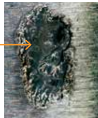
Electric arc pitting: Burns created by improper electric grounding while bearing is stationary.
