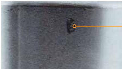
Electric arc pitting: Burns created by improper electric grounding while bearing is stationary.
