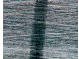
Damage from shock or impact.
