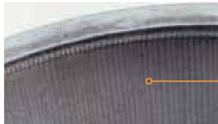
Fluting: Series of axial burns caused by electric current passing through the bearing while rotating.
