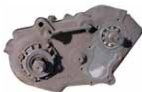
NP205 T/C figure-8 bolt pattern
