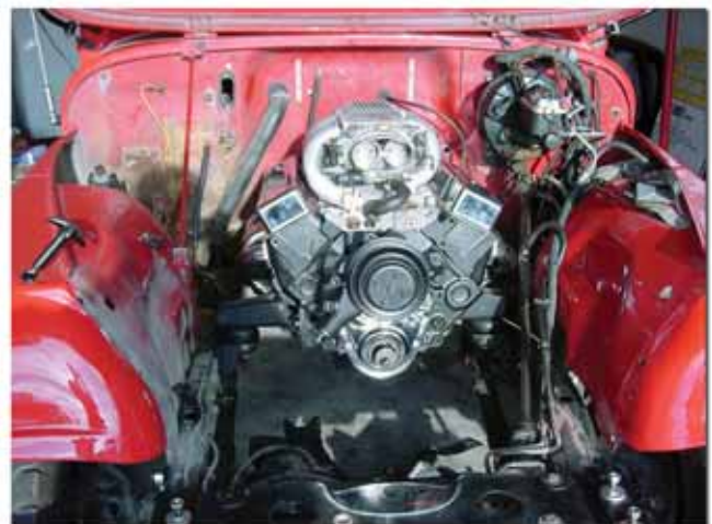
713089 bolt-in mounts with engine off-set
