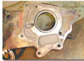
Small Hole transfer case (3-1/8")
