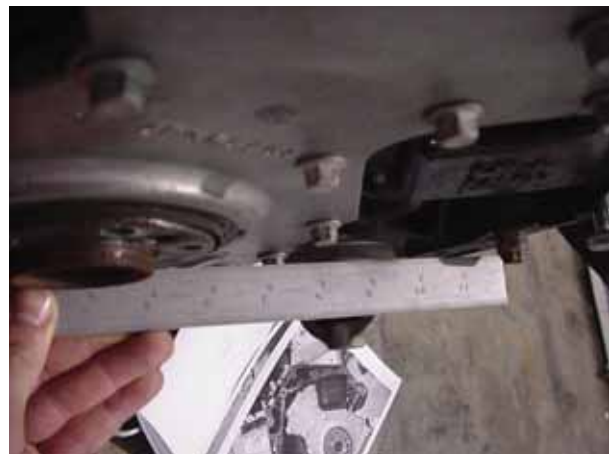
Crank stickout is almost flush with the back of the block
