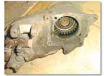
Large Hole transfer case (4")
