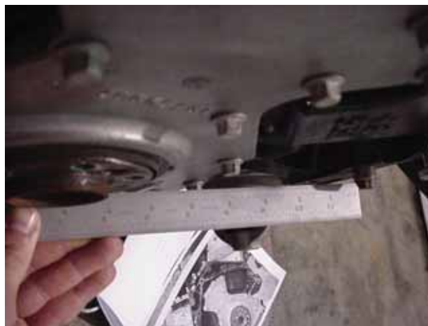
Crank stickout is almost flush with the back of the block
