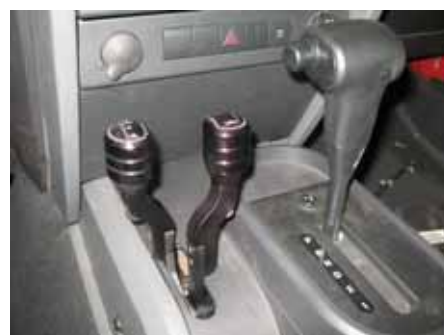
Jeep JK console (right) with the RubiCrawler twin stick shifter installed.
