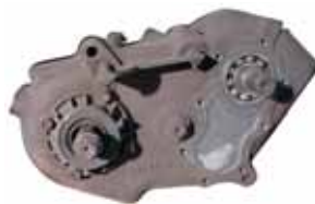
NP205 T/C figure-8 bolt pattern
