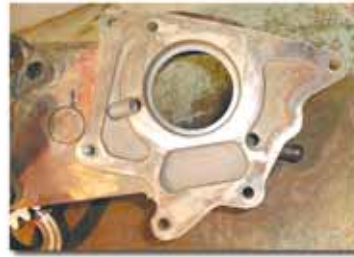
Small Hole transfer case (3-1/8")
