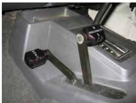
Jeep JK console (right) with the RubiCrawler twin stick shifter installed.
