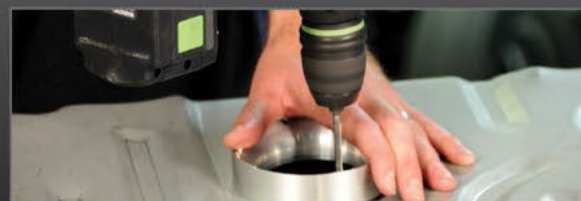
Use installation ring to locate mount holes,
