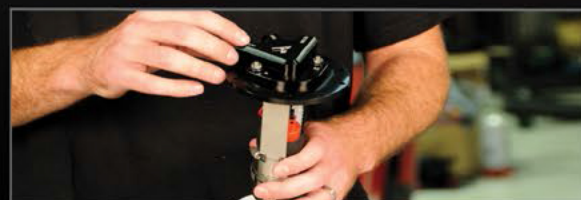
Install c-ring, pump, and tighten down
