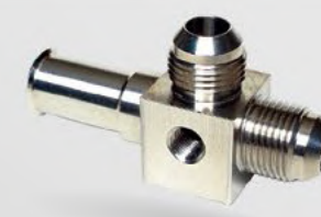
1/2" Female Spring-Lock / (2) AN-08 Male "T" (86-06 Ford Supply Line) #15102
