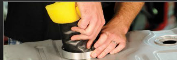
Insert foam inside the tank
