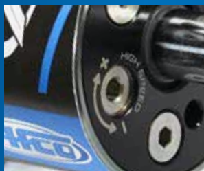
HIGH SPEED REBOUND ADJUSTMENT.
