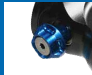
LOW SPEED REBOUND ADJUSTMENT.
