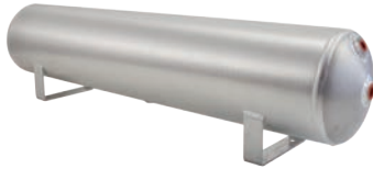
Aluminum 4 Gallon 11955 - Raw Finish 12955 - Polished (2) 1/4" NPT End Ports, (2) 3/8" NPT End Ports, (1) 1/4" NPT Drain Port Dimensions: 30"L X 6"D
