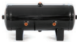
10980 - 2 Gallon (4) 1/4" NPT Ports, (2) 3/8" NPT Ports Dimensions: 6"H X 17" L
