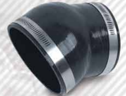
Angled Reducer 4" ID to 3.5" ID x 28° angle w/clamps P/N 130-435
