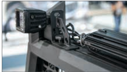
Topside track accepts LED lights and tie-down anchors (see pages 92 and 53)
