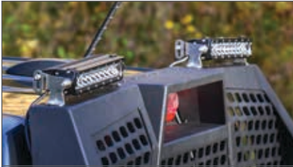
Slotted top edge accepts various LED lights (three 10" light bars recommended)
