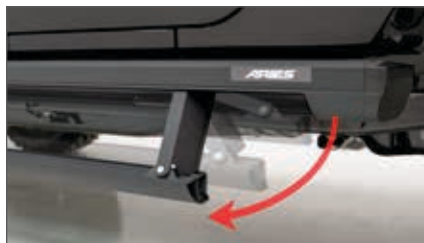
Housing shields retractable step, pivot points and electronics from the elements
