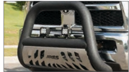
Two pre-drilled holes in the crossbar for mounting LED lights (see page XX for lights)
