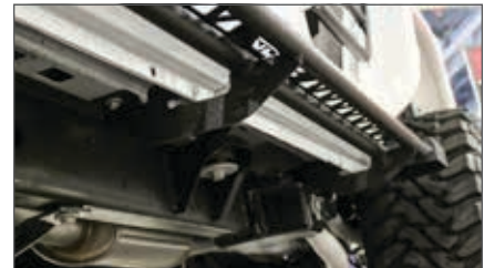
Pre-welded mounting brackets for increased rigidity and simpler installation
