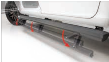
3" powered step automatically drops 8" when door opens, up to 15" below doorsill
