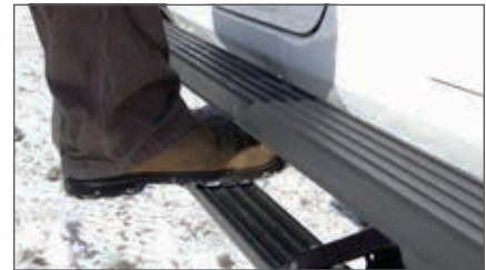
Integrated control module detects obstructions and eliminates pinch hazards
