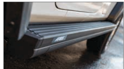
Contoured design helps protect the rocker panels from road debris and door dings
