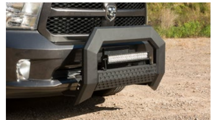
Crossbar without LEDs can be flipped to mount LED lights (see page 96 for lights)
