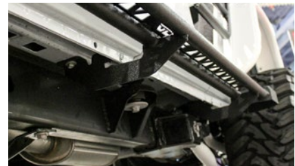
Pre-welded mounting brackets for increased rigidity and simpler installation
