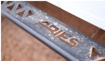
Double-tube layout and 3" wide top plate provide a solid step
