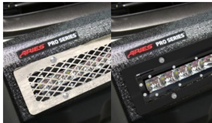
Interchangeable cover plate protects light bar and offers easy customization (see page 20)
