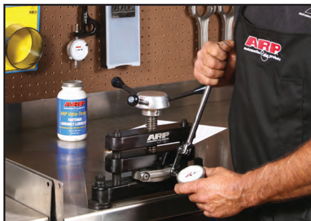
A rod bolt stretch gauge is one of the most important tools a serious engine builder can own. It's valuable in properly setting up a rod for resizing, obtaining the proper clamp load when installed. See page 127 for more information.
