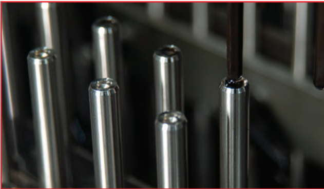
State-of-the-art EDM technology is used to perform special operations, such as hex-broaching head studs.
