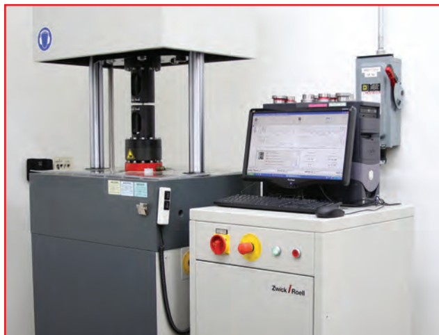
ARP has two highly sophisticated Amsler fatigue machines, which test fasteners through millions of cycles.
