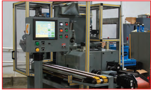
The Grinding Department is where all studs are centerless ground to ensure that they are perfectly concentric. As many as ten machining steps are required to achieve this level of accuracy.
