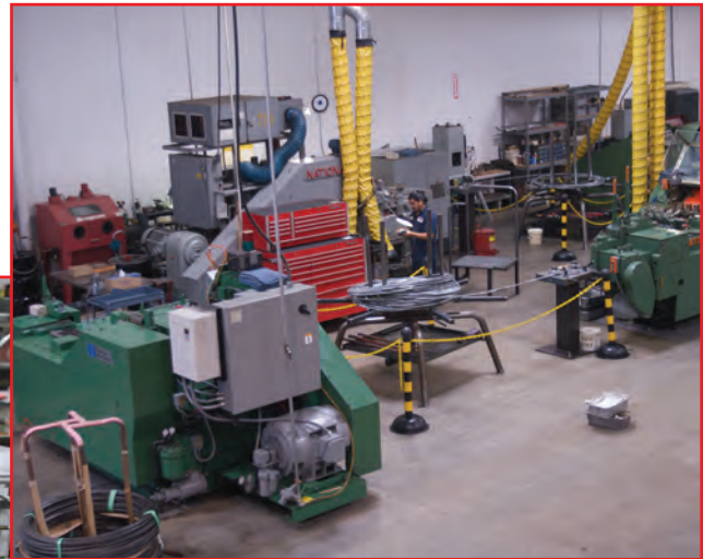
Powerful cold-forging equipment is used to make ARP's hex and 12-point nuts. Multi-stage dies are employed to precision-form the finished “blanks.”
