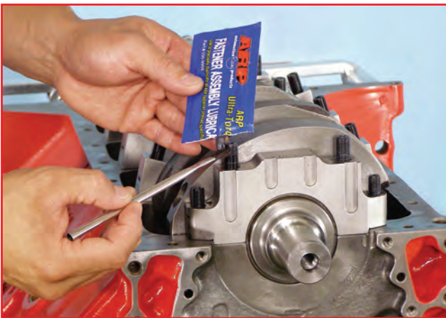
4. Install main caps, checking for binding and misalignment. Lubricate threads, nuts and washers with ARP Ultra-Torque fastener assembly lubricant before installation. Have the block align honed.
