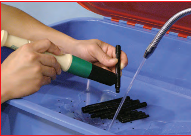
2. All hardware (and caps) should be cleaned and inspected prior to installation, looking for any shipping damage or defects.
