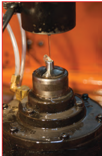
State-of-the-art EDM technology is used to perform special operations, such as hex-broaching the nose of a unique short-run fastener.
