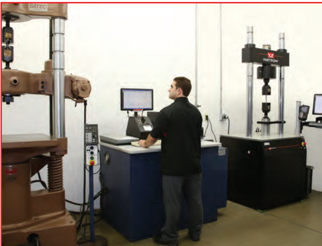
Two computer-controlled Instron tensile machines are used to determine the ultimate tensile strength of studs and bolts.
