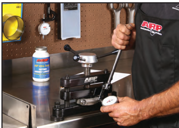
A rod bolt stretch gauge is one of the most important tools a serious engine builder can own. It's valuable in properly setting up a rod for resizing, obtaining the proper clamp load when installed in the engine, and monitoring the condition of the bolt while in use.
