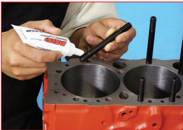
3. Since most studs extend into the water jacket, coat threads with ARP thread sealer and screw in hand tight ONLY .
