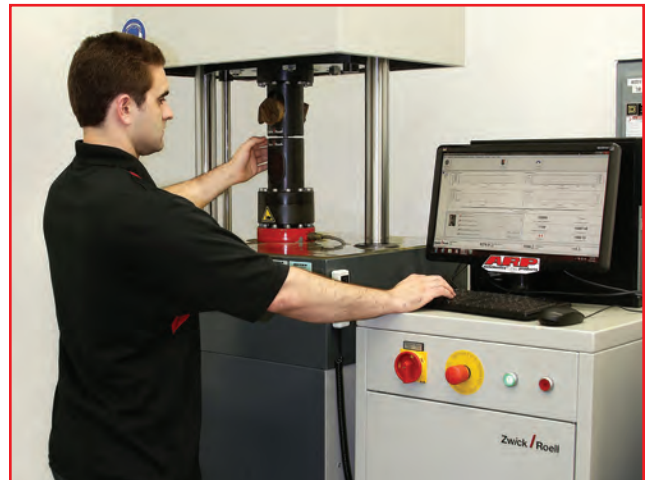
ARP has two highly sophisticated Ansler fatigue machines, which test fasteners through millions of cycles.
