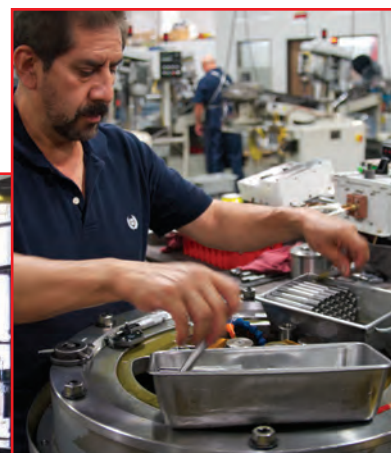
ARP performs the thread rolling operation after heat-treating, which results in a fatigue strength up to 20 times higher than fasteners with threads rolled prior to heat-treatment.
