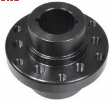
Hub For SBC 6 Bolt 3/8-24, Chrysler Front with 3/16 Keyways (Part #916136)
