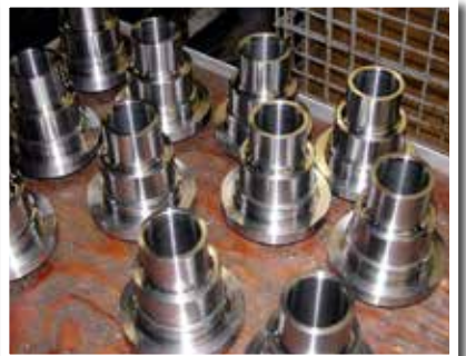
Type 2: Dampers with a separate inner shell
