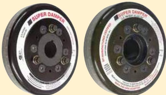
Typical SBC OEM style flat faced hub
