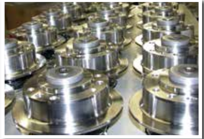
Type 1: Dampers with the crank hub and inner shell as one combined part (Figure 1)
