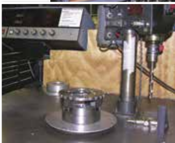
Precision balancing of heavy duty carriers
