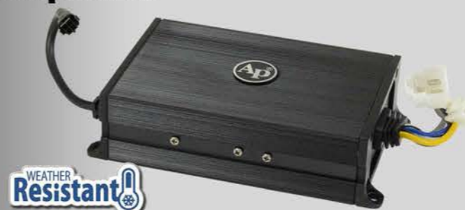
Rubber cover seals controls on side panel
