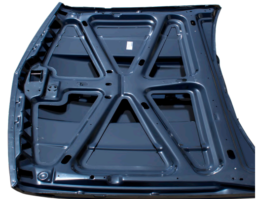
Original Style Bracing
