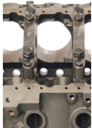
NODULAR IRON 4-BOLT SPLAYED MAIN CAPS
