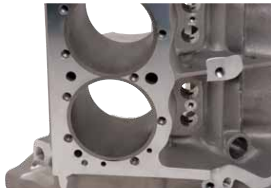
SLEEVES WITH THICK REGISTERS INSTALLED ASSURING PROPER RING SEAL
