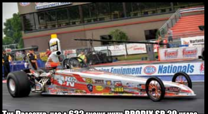
THE DRAGSTER HAS A 632 ENGINE WITH BRODIX SR 20 HEADS, BRODIX ALUMINUM BLOCK, AND A BRODIX INTAKE MANIFOLD.
