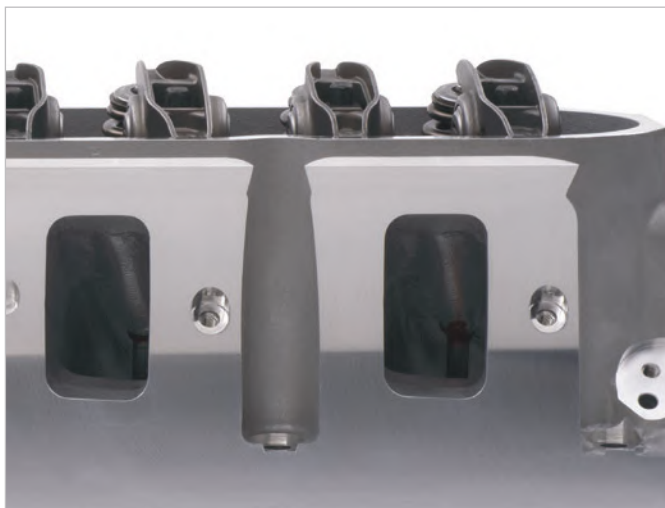
C LS7 Intake Port and Bolt Pattern
