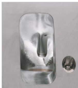
LS3 CNC-Ported Cylinder Head Assembly (intake detail) A
