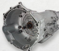
19368611 SuperMatic™ 4L65-E Four-Speed Automatic Transmission (remanufactured) Electronically controlled four-speed overdrive transmission. Suitable for engines producing up to 430 lb.-ft. of torque.
