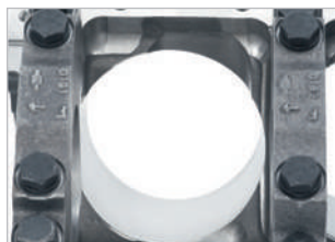
Top: Splayed Main Cap C Bottom: Machined Bottom
