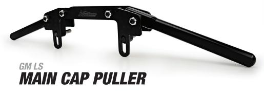
The LS Engine Main Cap Puller is specifically designed to fit LS engines. This sturdy tool makes the job of removing the doweled main caps quick, safe and easy. In one smooth motion, caps are removed and held tightly so they don't fall and become damaged - no prying, hammering or damaging dowels required.
