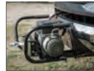
Allows a winch to be easily mounted to a receiver (31009)
