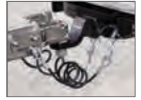
Safety cables in use
