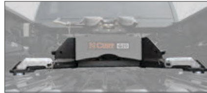
Ram legs installed in a long-bed truck with Q20 head (16045)
