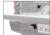
7' routes socket into rear of the truck bed
