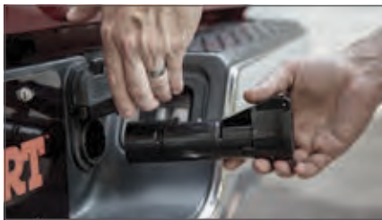
Insert Echo™ between the vehicle and trailer
