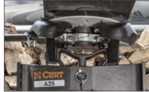
Adds a buffer between 5th wheel head plate and kingpin box
