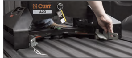
Step 2 - Close the anchor levers to lock the 5th wheel into place
