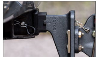
Reduces the receiver tube opening to fit smaller shank sizes
