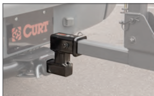
45794 provides added ground clearance
