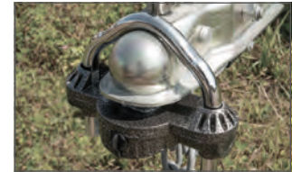
Universal design fits all coupler types and styles (23659 shown)
