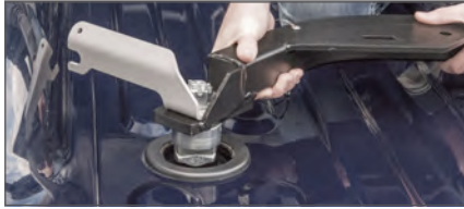
Step 1 - Drop OEM product into the truck bed puck system
