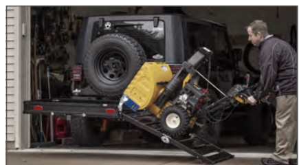
Built-in ramp for easy loading of scooters, push mowers, snow blowers and more
