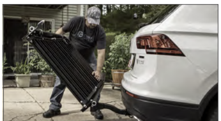
When not in use, carrier folds up for convenient parking and storage
