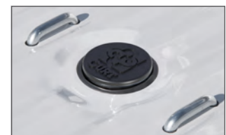
Install the hole cover to protect the ball from the elements
