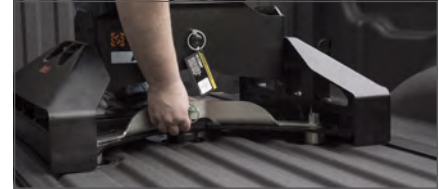
Step 3 - Secure levers with attached safety pins and you're ready to hitch up your trailer
