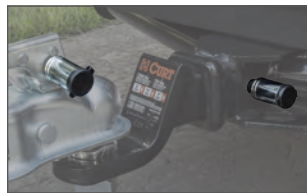
Watertight dust caps prevent internal corrosion
