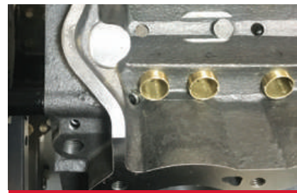
1/2" NPT Oil Feed / Removed Rear Crossover
