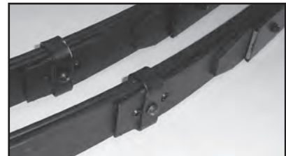
Tapered leaf springs with anti-friction pads
