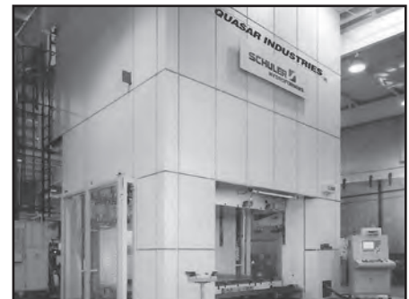
The large hydraulic press where the framersails are made
