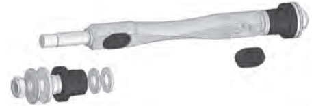
Rendering of the upper control arm cross shaft
