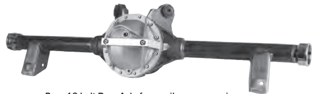
Bare 12 bolt Rear Axle for a coilover conversion with optional DSE aluminum support cover
