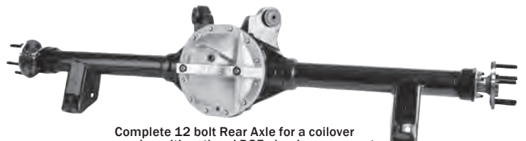
Complete 12 bolt Rear Axle for a coilover conversion with optional DSE aluminum support cover and optional powder coating
