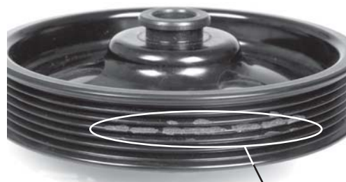
Road Debris Damage
