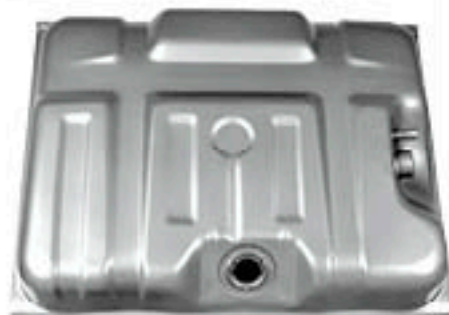
T3002 1973-78 Gas Tank Rear Mount, Vent Pipe Towards Rear, 19 Gallons
