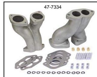
Extra Thick Aluminum Manifolds
