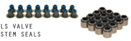
The valve stem seal allows a carefully defined amount of engine oil from the cylinder head into the combustion chamber allowing a necessary lubrication of the rotating valve stem in the valve guide.
