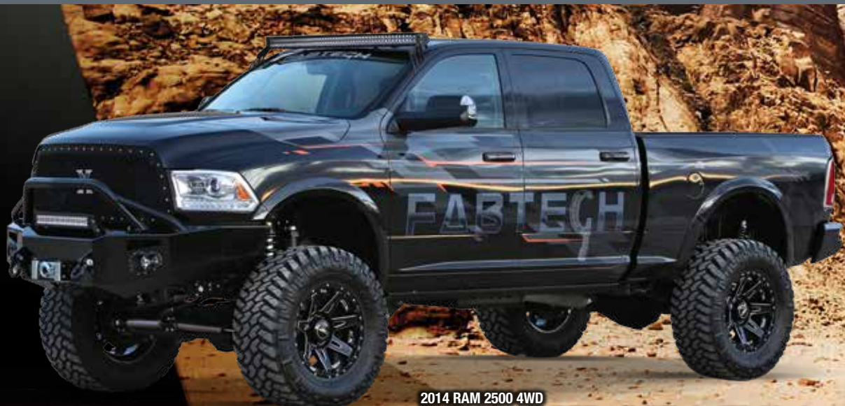
2014 RAM 2500 4WD 7" 4 Link System 38x13.50 Tires 20x10 Wheels w/5" Back Spacing
