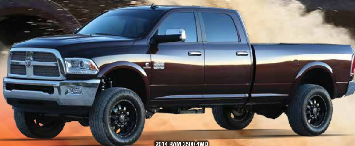
2014 RAM 3500 4WD 5" Radius Arm System 37/12.50R20 Tires 20x10 Wheels w/5" Back Spacing
