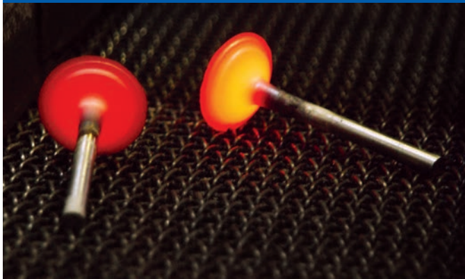
▼ Valves after the forging process
