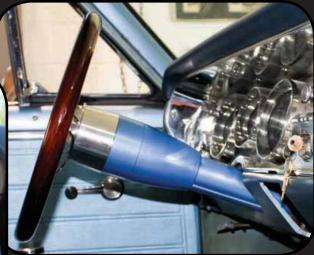
FR20143 67 & Prior Wheel Adapter installed on a 66 Chevelle Steering Column.
