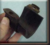
Utilize your original dash support (Note: you must first place the shim that is included in your installation kit between the support and the column to ensure a tight fit)
