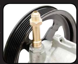
LS3 Power Steering Pump Extended AN Fitting Part No. - FR1634 Corvette-Style "Transverse Compact" Low-Flow Pump (5/8" Shaft Size) FR1571 This Transverse Compact Pump is ideal for street rods and features a bearing design and a flow of 2.4 to 2.8 gallons per minute. Polished version also available. Remote Reservoir (FR1614) required.
