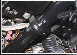
Install the upper portion of the new Flaming River® Mounting Clamp into the stock location.
