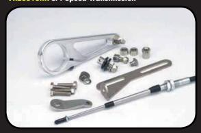
Lokar Cable Shift Linkage kit Lokar Cable Shift Linkage is the ultimate answer to clearance issues. The cable allows you to route around transmissions, exhaust, cross members and brake pedals. Can be used on either side of the column. The cable has a Teflon-lined black housing with stainless inner-wire, measuring 5 ft. in length. Ready-to-install hardware and brackets included in kit - no cutting or measuring. FR20010CBL
