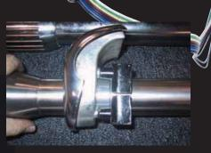
Install the original dash bezel and column mounting bracket over the new split ring spacer onto the new Flaming River® Tilt Column.
