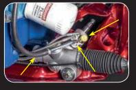
Fitting Adapter Kit to attach to your original pump. Includes return fitting and hose and pressure line adapter.
