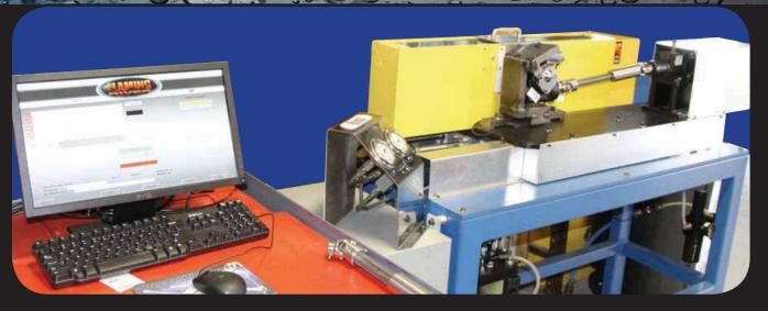
Each Flaming River manual steering box is tested for proper steering torque and bearing adjustment... Flaming River Certified!
