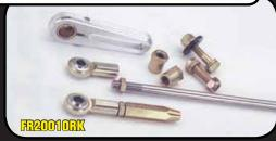
Lokar Billet Aluminum Linkage Kit This adjustable kit connects and aligns a gearshift arm to a GM automatic transmission. Includes adjustable billet aluminum arm, two adjustable Heim-style connectors, a shift rod, and all mounting hardware.
