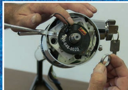
4. Place the final 3/16" aluminum spacer over the column shaft and down to the canceling cam.
