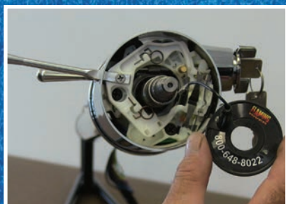
3. Then, slide the Canceling Cam over the column shaft and canceling cam spring.
