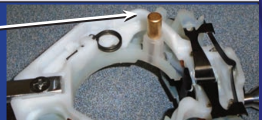
5. When installing your steering wheel adapter, tighten the retaining nut to 50 ft lbs.
