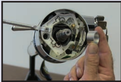
1. Install the large 5/8" aluminum spacer over the column shaft.
