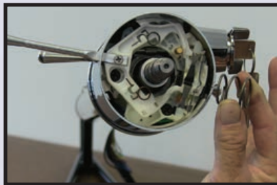
2. Next install the Canceling Cam Spring over the column shaft and down to the 5/8" aluminum spacer.
