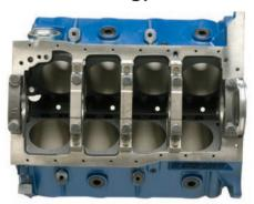
"Using a BOSS 351 block as a foundation became a no-brainer. The block provides about the best bang for the buck anywhere and hardly costs any more than a stock Windsor block that has been fully machined and blueprinted. But the BOSS block still has some advantages over that, namely, it's cast using diesel-grade iron, which exhibits a much greater tensile strength than a stock casting. Plus, there is extra meat in all the critical stress areas.
