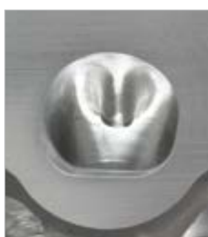
LS3 CNC-Ported Cylinder Head Assembly (exhaust detail) A
