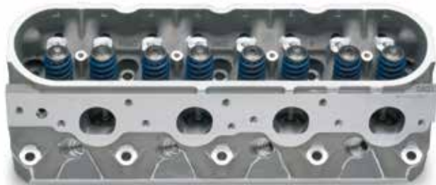
LS3 CNC-Ported Cylinder Head D
