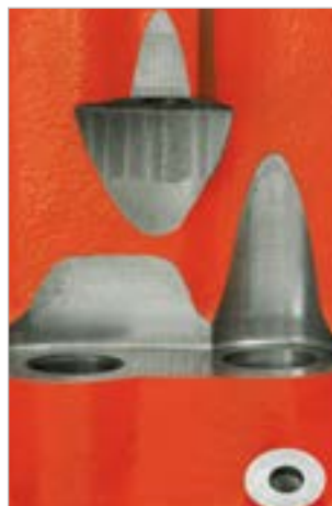
A Machined Lifter Valley Detail
