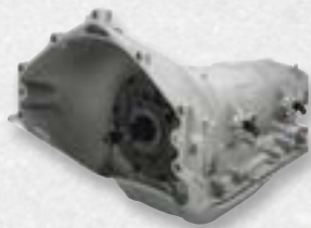
19300175 SuperMatic™ 4L85-E Four-Speed Automatic Transmission Features five-pinion gearsets, heat-treated stator shaft splines, induction-hardened turbine shaft, seven-plate clutch and specific valve-body calibration. See page 364 for torque converter applications.
