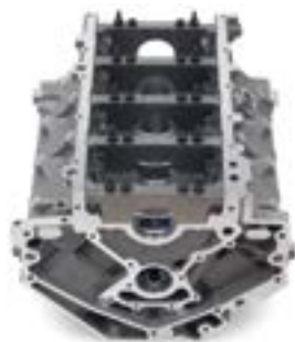
LS3/L92 Aluminum 6.2L Bare Block (bottom) B
