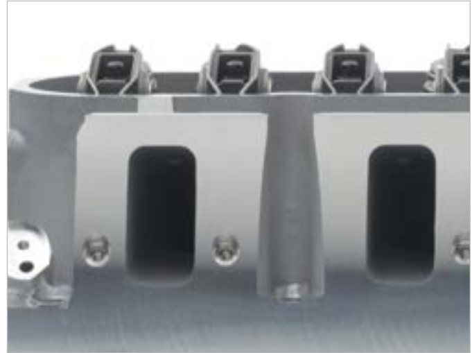
B LS3 Intake Port and Bolt Pattern
