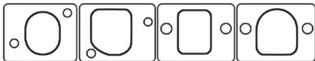
Not all flanges are round or square port. There is a variety of shapes and sizes. Flange gaskets must match header port shape and size to avoid blowout or warped flanges.
