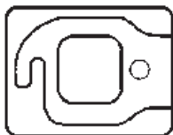
Correct gasket for square port Header, only if same size and shape as Header flange.
