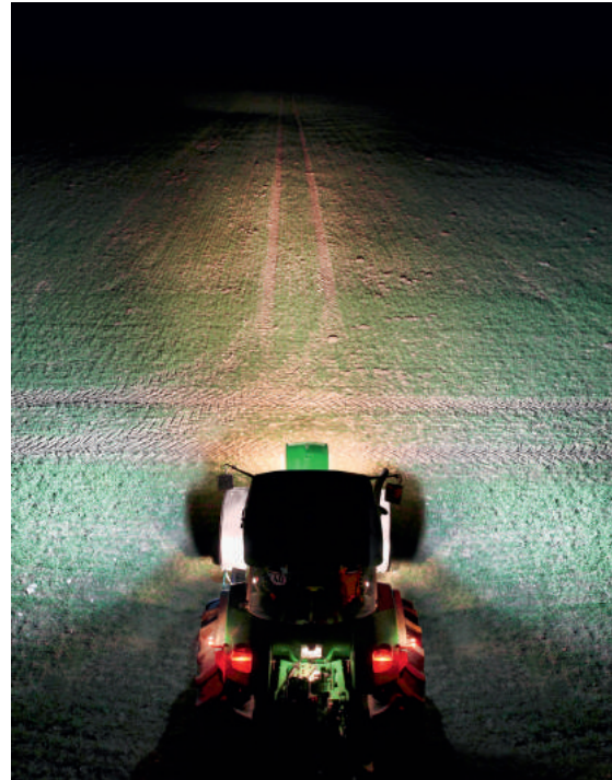
Upgrade Option 1: 4 x Halogen Work Lamps, 2 x LED Work Lamps Alternator load 22.0A
