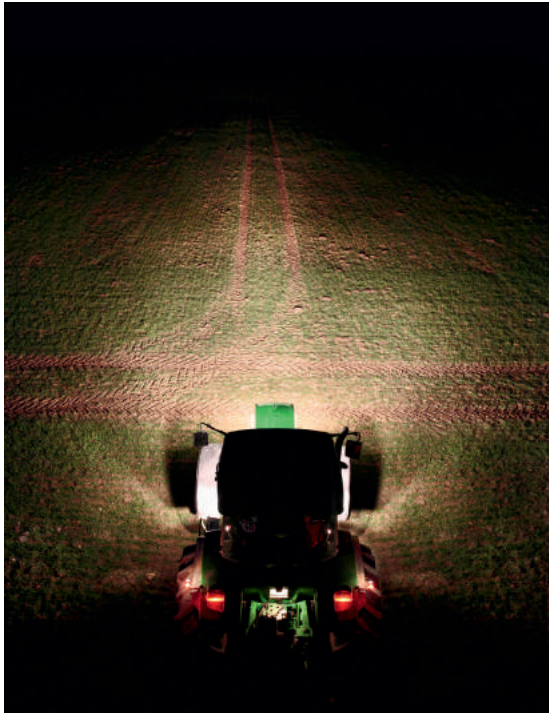
The Past: 6 x Halogen Work Lamps Alternator load 27.5A
