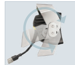
Multi-adjustable Trunnion bracket ensures accurate and stable aiming in a high vibration environment in all assembly positions. Bracket locates the axis of rotation in the centre of gravity.
