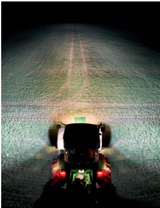
Upgrade Option 2: 2 x Halogen Work Lamps, 4 x LED Work Lamps Alternator load 16.5A
