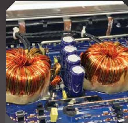
Twin turbo power supply toroids in a PWM MOSFET power supply design
