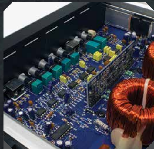
Accu-Cross™ crossovers and adjustments for sound shaping
