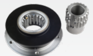
Quick Release Steering Hub with Centering (pg 65)
