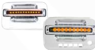
F-150/F-250 LD 04 - 08 LED DOOR HANDLE, FRONT CHROME (2PS/SET) AMBER LED/SMOKE LENS RH NO KEY HOLE, LH KEY PAD FLA04SF1
