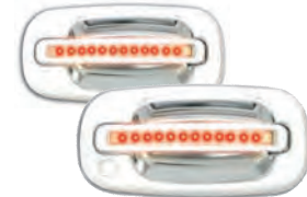
SILVERADO 99 - 06 LED DOOR HANDLE, FRONT CHROME (2PS/SET) RED LED/CLEAR LENS, RH NO KEY HOLE CLR99C18F1
