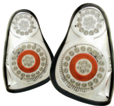
MONTE CARLO 00 - 05 LED TAIL LAMPS CRYSTAL CLEAR, RUNNING & BRAKE: UPPER & LOWER OUTER RING TURN: UPPER & LOWER INNER LEDT-344C
