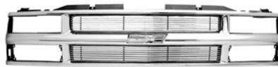
CHEVY PU/CK 94 - 99 BILLET CONVERSION GRILLE, 4MM CHROME, RECESSED FOR OE LOGO CWGI-9498CK4
