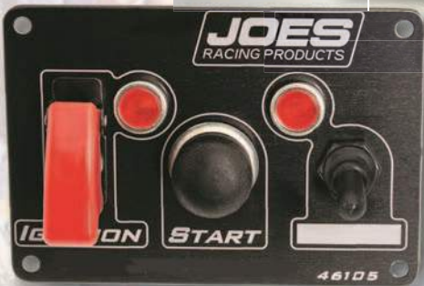
#46105 Panel-Flip Up/Ign./ Start Button/ Accessory Switch - w/ Light & Rubber Sealant
