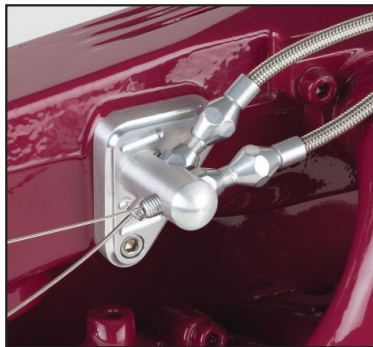
'88 and earlier throttle body end fitting shown
