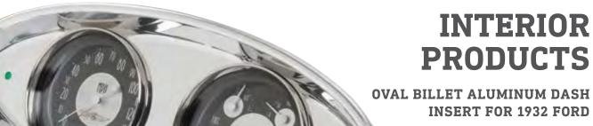
Oval Billet Aluminum Dash Insert features recessed face design. Designed to fit original 1932 Ford dash. Styles available for VDO, Classic Instruments, Ford Masterpiece and Auto Meter Gauges. Gauges mount from back of insert. Two green 12 volt turn signal LEDS and one red 12 volt high beam LED included. Holding clips and screws included. Gauges not included. Available in brushed or polished. Dimensions: 11-13/16"
