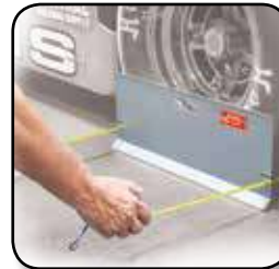
Magnets hold tapes in place during use.
