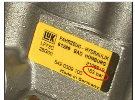
LuK power-steering pump with pressure control valve
