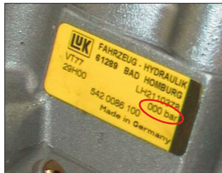
LuK power-steering pump without pressure control valve
