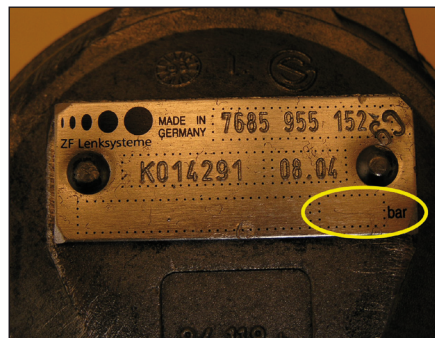
ZF power-steering pump without pressure control valve
