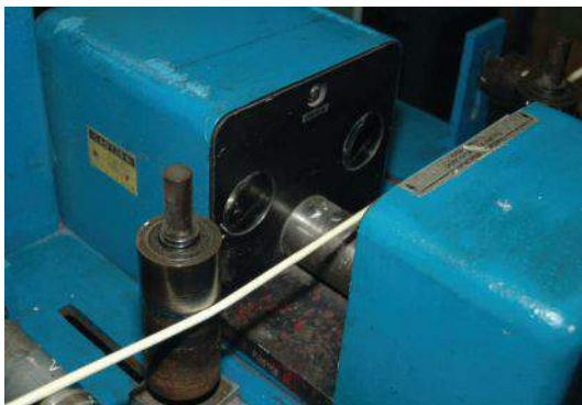
An optical laser measuring device keeps constant measurement on the completed wire as it comes to the end of the line. The machine operator must maintain the measurement within a specified amount and adjust as necessary.
