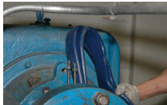
The outer silicone material is fed through the machine in the same fashion as the center core cover, eventually making it's way onto the wire and completing the forming process.
