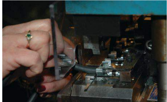
Each wire is hand fed into a crimping machine that automatically feeds terminal ends through it, while an operator feeds the previously stripped back wire in, finally ending up with a crimped terminal on the end.
