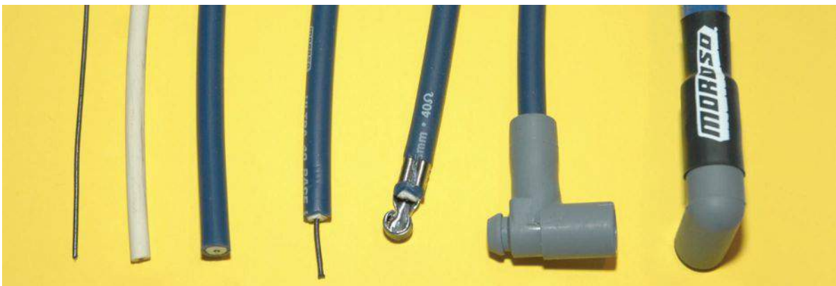
The manufacture of Ignition Wire requires several different steps: first, the center conductor (1) has EPDM (Ethylene Propylene Diene Monomer) rubber material formed around it (2). The wire is then re-fed into the machine where the outer silicone covering is formed and printed with the type of wire it is (3). The completed wire is then stripped back (4) and the terminal ends are crimped on (5). The plug boot is installed (6) and finally, for race applications, a silicone-jacketed fiberglass sleeve is slipped over the assembly and a shrink sleeve installed (7).
