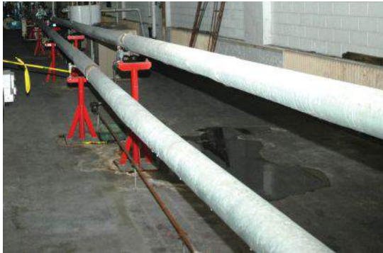
The wire travels 250 feet through these long tubes on the right in order to cure and cool the wire after manufacturing.
