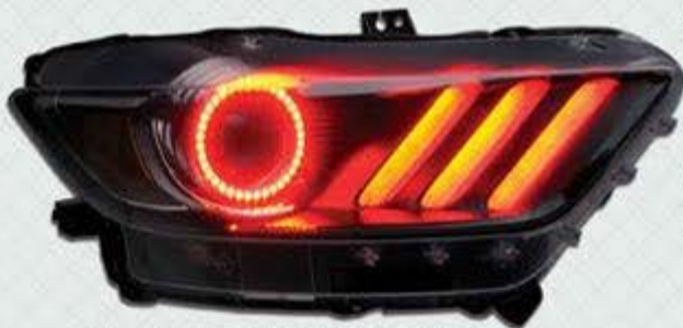
RGB 5050 Concept SMD strips installed as Daytime Running Lights behind the OEM diffusers.
