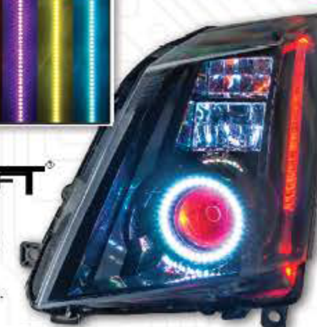
RGB 5050 Concept SMD strips installed as Daytime Running Lights behind the OEM diffusers.
