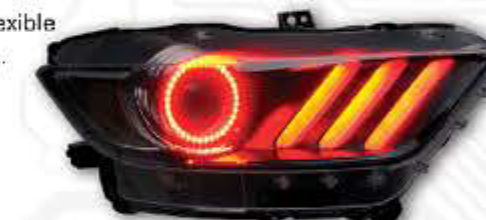
ColorSHIFT Concept SMD strips installed as behind the factory diffuser lenses.
